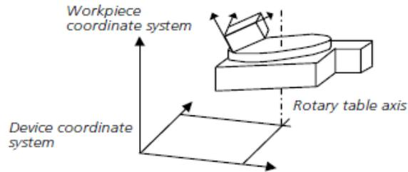
All features and coordinate systems are computationally rotated around the RT axis when the rotary table turns.
